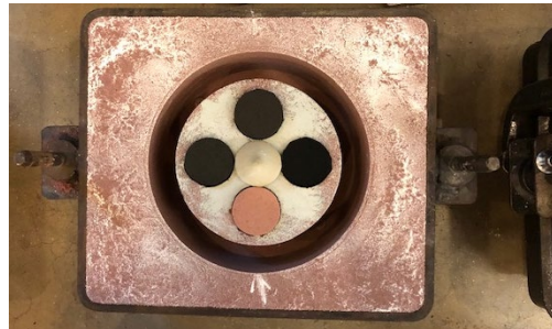
Figure 10. Drag mold with specimens on coreprints.
