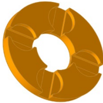
Figure 7. Shell sand core used to deliver molten metal over the specimen surfaces.
