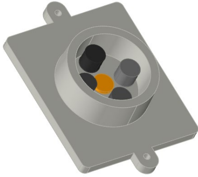
Figure 6. Drag side of matchplate pattern.
